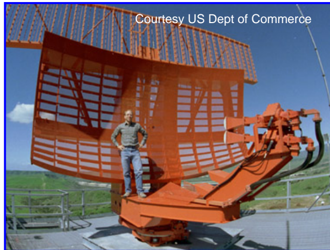
Airport Surveillance Radar
